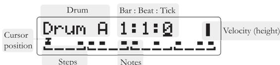
In the top line, the screen indicates that Drum A is being edited in Step mode. The cursor is at bar 1, beat 1, tick 0, shown as 1:1:0.
