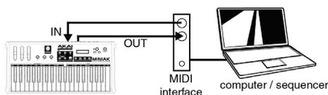
For this setup, switch the MINIAK's Local Control setting to OFF (in the **[CONFIG]** settings).
