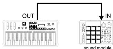
For this setup, ensure that the MINIAK's Local Control setting is ON (in the **[CONFIG]** settings).
