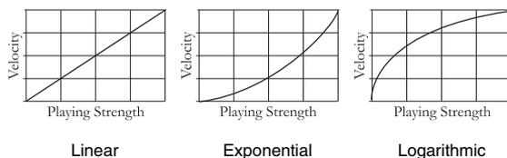
Press the DATA DIAL to edit the velocity curve. Turn the DATA DIAL to select a new curve. Press the DATA DIAL again to accept the curve setting and return to the main config menu.
